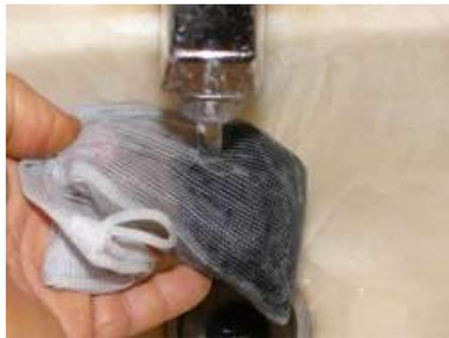
Slip the bag into the filter housing, fold the rest of the bag down on top.
