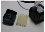
Take off the grid, underneath is a foam filter and another black cover with a round hole that you can pull off, making the white impeller visible. Gently remove the impeller making sure not to bend or damage the white plastic part. Hit the pump against your hand so that anything that might be lodged inside has a chance to come out.
