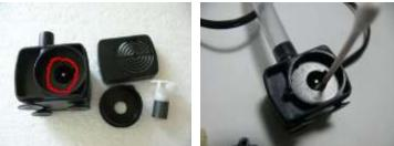
Then rinse everything, clean the hole with a Q-tip, being very careful not to bend or damage the impeller axle (circled in red in the picture). If very slimy or calcium encrusted, soak in a 1:10 solution of vinegar and water.
